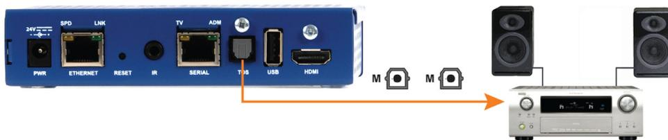
**TOS** – Use a standard TOSLINK cable to connect the 2 channel PCM or Bitstream audio output to an external audio system if required.
