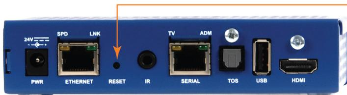
You can reboot the receiver by pressing a pin or the end of a pen into the **RESET** port. You can also return the receiver to the factory default settings.
