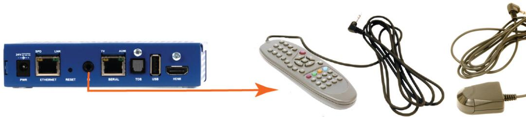
**IR** – Connect the tethered remote control when control with the IR handset is not possible or desired.
