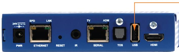
An external storage device (FAT32 format) can be connected to the USB port. The storage device can be used to hold items such as video content and playlists to provide failover support, additional fonts, and html content for digital signage.
