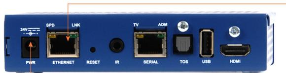
**POE** – The receiver can be powered through the network interface by Power over Ethernet (PoE) using any LAN Switch or Mid-span device meeting 802.3af PoE specifications.
